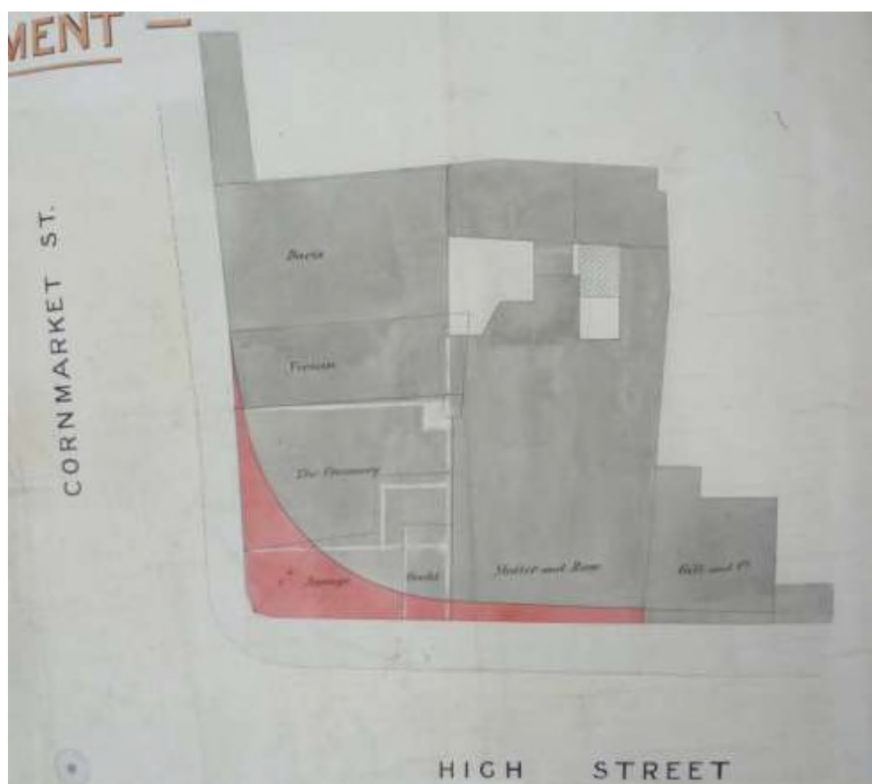
Extract from an Oxford Corporation plan of "Carfax proposed improvement", 22 December 1899. The curved corner that the corporation wanted to create depended on Lloyds Bank setting its new building – which would replace Slatter & Rose's shop – back by several feet. City Engineer's strong room plan 6081, courtesy of Oxford City Council.
